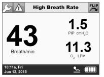
**4** The top of the touch screen should display the High Breath Rate alarm, and you should hear a sequence of three tones indicating a medium-priority alarm or vibrate.
