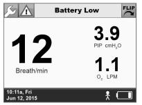
4 The top of the touch screen should display the Battery Low alarm and you should hear a sequence of three tones indicating a medium-priority alarm or vibrate.
