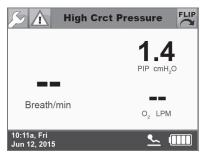
**5** Within a few seconds the top of the touch screen should display the High Circuit Pressure (High Crct Pressure), and you should hear a sequence of two sets of five tones indicating a high priority alarm.
