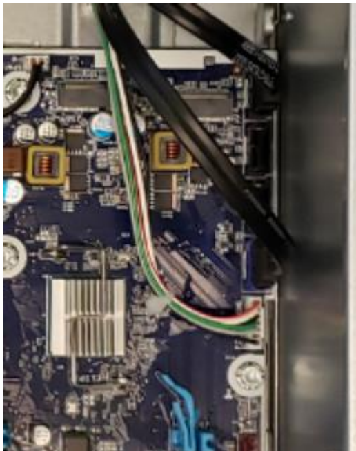
Zoom View of data cable connections
