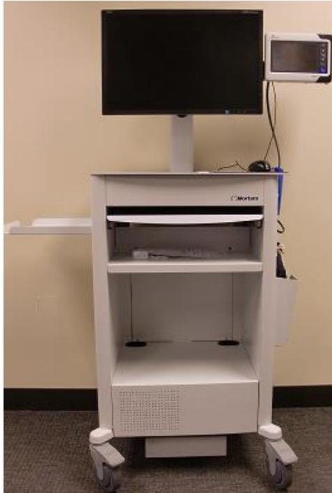
Finished Cart with the Z200+ Thermal Writer configuration, 24" LCD, SunTech Tango M2 BP monitor and Computer components installed.
