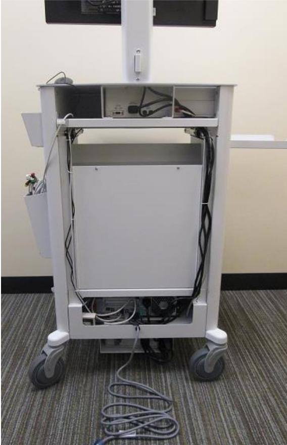
Organize the cables neatly at the cart back, routing them through the cable channels, secured with nylon tie wraps.
