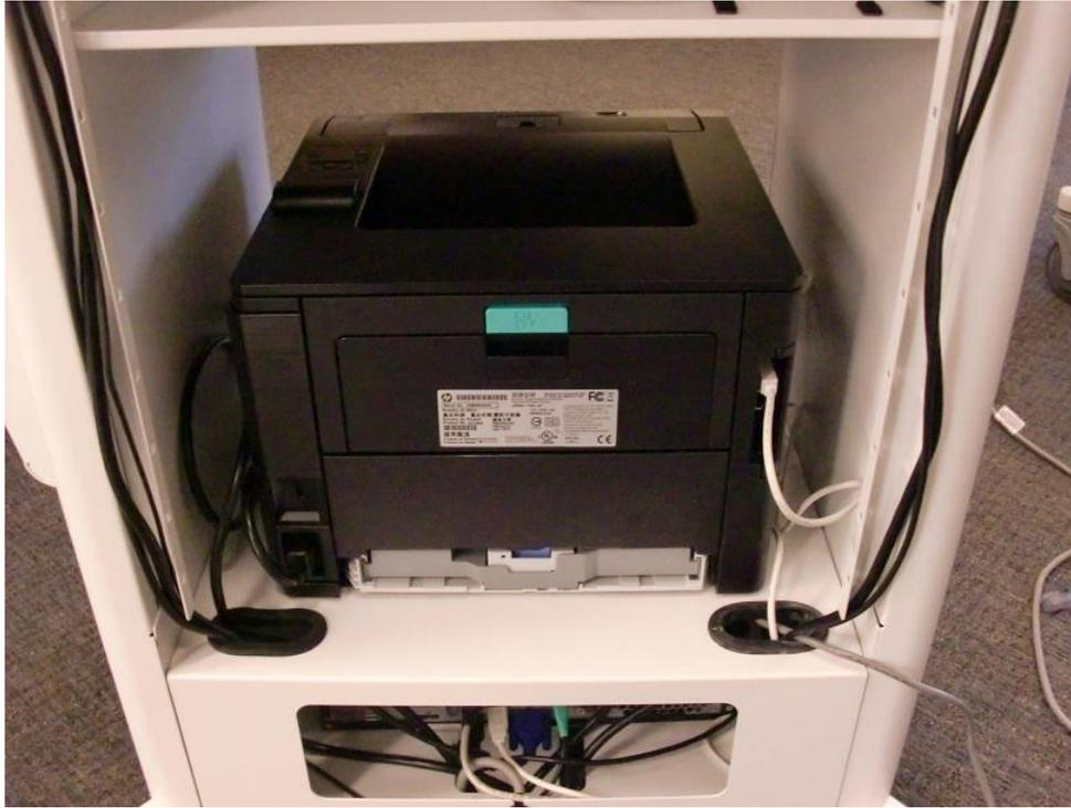
The cart back panel has been removed for easy access to the printer back during installation. This is done via removal of two M4 x 6 mm screws at the top of the panel.
