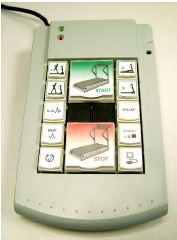
Connect the USB cable from the remote keypad to any available USB port on the back of the CPU.
