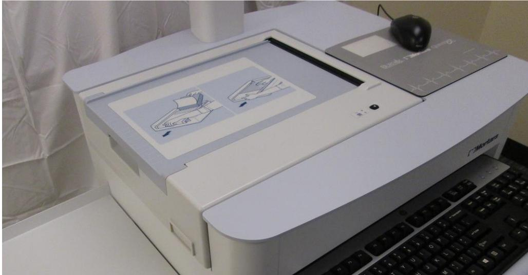
Route the power cable for the Z200+ thermal writer through the channels and cutouts to the isolation transformer and the data communication cable (either a USB cable for Z200+ v2, or a network crossover cable for Z200+ v1).
