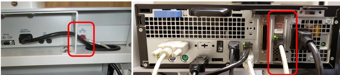
If using a Z200+ with an integrated network (LAN) connector, connect the ethernet crossover cable from Z200+ thermal printer to secondary LAN card on the PC following the channels and cutouts. The LAN port used for the Z200+ should be labeled “Z200+” from the factory. (LAN connections shown above)
