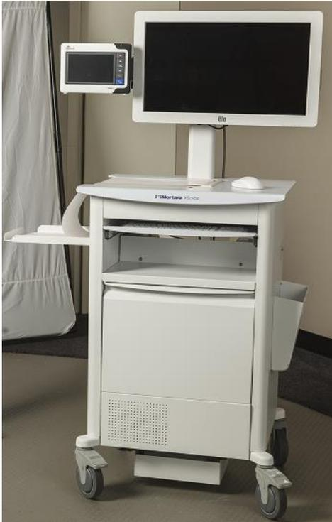
**Figure 3 Example of a Stress Cart with a Windows LaserJet Printer, Tango M2, and Touch Monitor**
