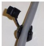
Place the plastic cord protector onto the main AC Power Cord as shown.
