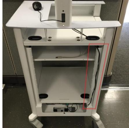
Route the data cables on the right-hand side as shown and the AC power cables through the hole on the left-hand side of the stress cart.
