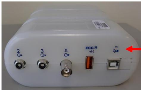
The Trigger Module back has (2) **currently non-functional** analog out connections, an ECG B connector for a WAM-UTK connection, (1) TTL output connection, and a USB PC connector.
