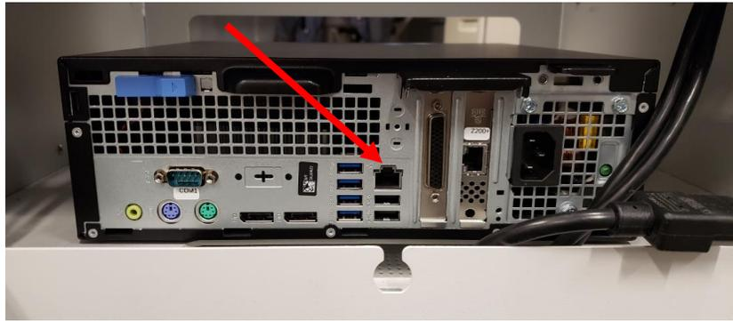
Connect the LAN isolator adapter to the Network Port (RJ45 connection) shown above right and connect the institution LAN cable to the isolator. Then use the Velcro provided to attach the isolation adapter in a convenient location, as shown above left.
