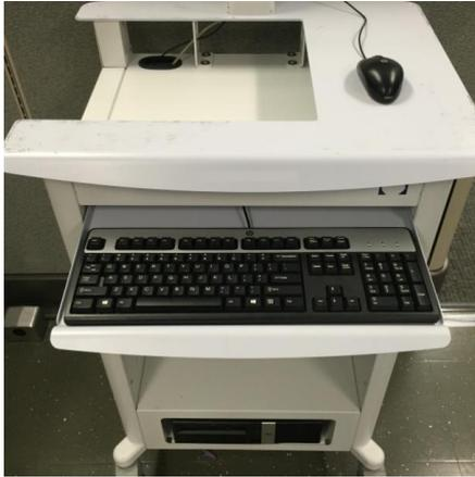
Place the keyboard on the tray. Route the cable through the back of the drawer and attach the connector to the computer back.
