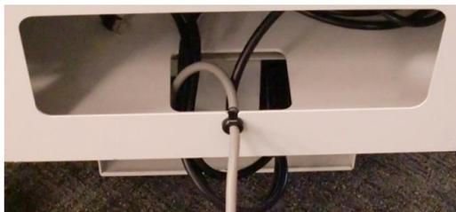
Insert the cord protector into the power cord cutout on the stress cart.
