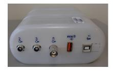
The module back includes two non-functional analog output connectors ( $\Rightarrow$  2 and  $\Rightarrow$  3) and one TTL output ( $\square$  $\Rightarrow$ ) connector.
