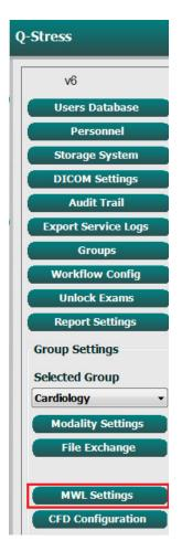
The MWL settings are for filtering the MWL items Q-Stress Server seeks from the MWL SCP.
