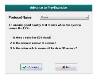
**NOTE**: The noise cancelling Source Consistency Filter (SCF) is very effective but MUST LEARN EACH PATIENT'S OPTIMAL ECG CONFIGURATION WHILE IN THE POSITION OF EXERCISE WITH A NOISE FREE SIGNAL.
