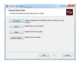
**Server:** This option allows for installations using multiple networked computers with the Database Server functionality loaded onto a separate computer or a Server hardware platform.
