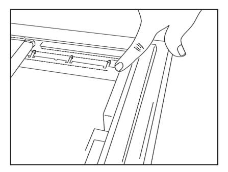
2. The paper-tray spacer should be parallel to the rear wall of the writer tray as pictured above.
