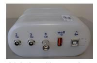
The module back provides two analog output connectors ( $\Rightarrow$  2 and  $\Rightarrow$  3 are currently nonfunctional) and one TTL ( $\Rightarrow$   $\vdash$ L) output connection.
