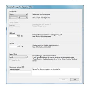
**Server Address:** This setting is grayed out when the Database Server functionality will be installed on the local PC, but will become an active selection when the modality will be accessing a remote Database Server.
