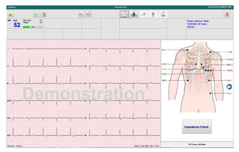
Check ECG waveform quality and lead placement, and then select **Impedance Check**.
