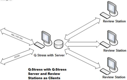
A central dedicated Q-Stress Server can be hosted on server hardware with any number of Q-Stress workstations as clients. Any 3<sup>rd</sup> party information system can exchange XML and PDF files with the Q-Stress Server.
