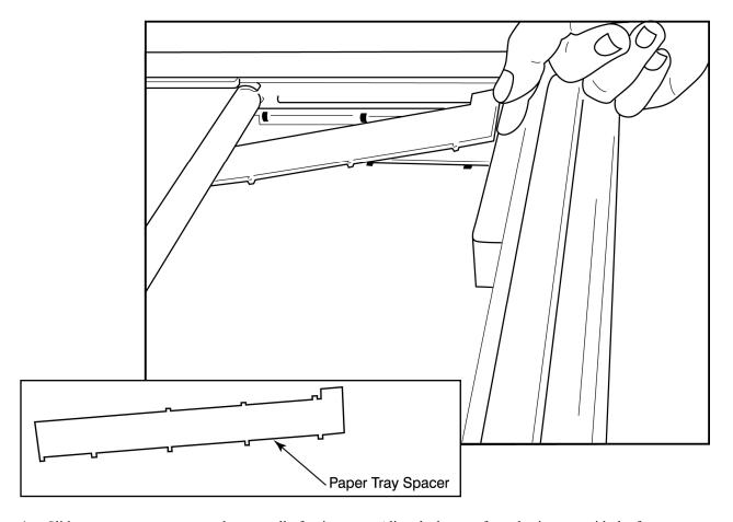
1. Slide paper-tray spacer towards rear wall of writer tray. Align the bottom four plastic arms with the four openings in the base of the writer tray. Similarly, align the top 3 plastic arms with the three openings on the rear wall of the writer tray.
