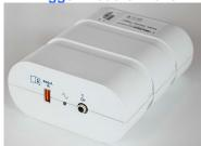
Q-Stress AM12Q Front End may be connected to ECG A USB connector on the module front. One analog output connection ( $\Rightarrow$  1) is also on the front.
