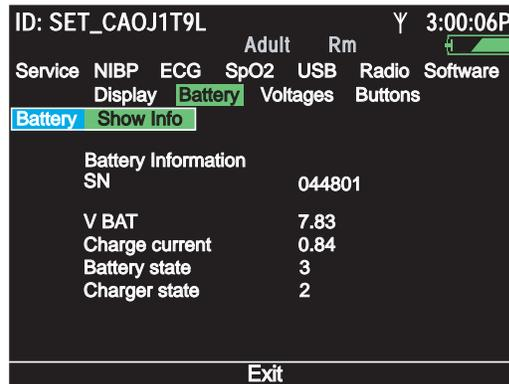
10. Verify that the charge current is between 800 mA and 1100 mA and that the charger state is 2.
