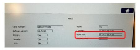
The MAC address contains 12 characters, where the first 6 characters are used to determine the model of the WLAN module installed. The remaining 6 digits will change with each device.
