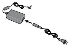
2. Locate the power connector on the vision screener and connect the power supply.
