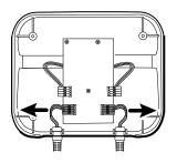
f. Lift and remove the handle cables from the front handle housing.
