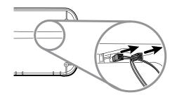
k. Push in the snap tabs and then remove the cradle assembly by pushing outward.
