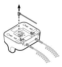
c. Remove the rear housing by removing the four large Phillips screws.
