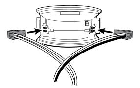
I. Snap the handle cradle assembly into the front housing. Make sure that the cradle assembly tab and the beveled edge are at the top of the housing.
