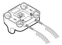
d. Lift and remove the rear housing.
