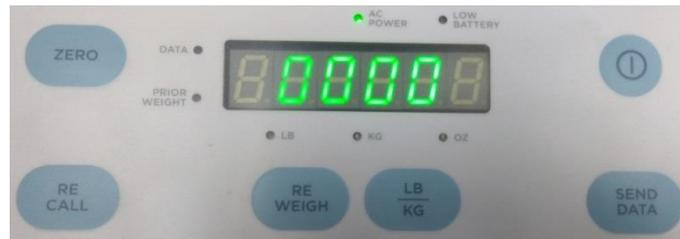
2. Enter PIN number "9821" into the Scale. (Press 'RE WEIGH' button to increment the value, 'RECALL' button to decrement the value, 'LB/KG' button to shift to the next digit or to confirm the PIN).
