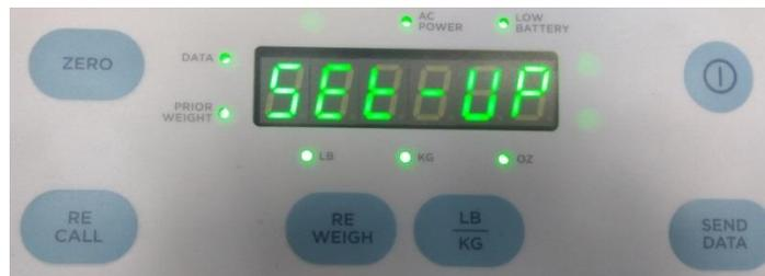
4. Press the **"LB/KG"** button until **"SOFT"** is displayed. Press **"LB/KG"** one more time, the firmware version will be shown (U X.X.X). (See below reference).
