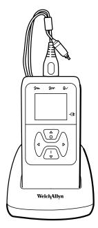
Place the screener in the cradle to charge the device or to connect to a computer for communication with the Welch Allyn Data Manager (data manager). You can also charge the device or connect to a computer directly from the screener.
