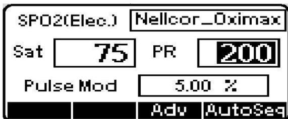
22. [CVSM] Verify that Saturation level is 75% ±1% and Pulse Rate is 200 bpm ± 2 bpm [Pass/Fail]
