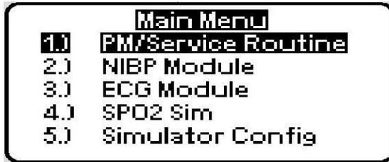
13. [AccuSim] Press the “Scroll up/down” button to select the “ECG Module” and press “Enter” to launch
