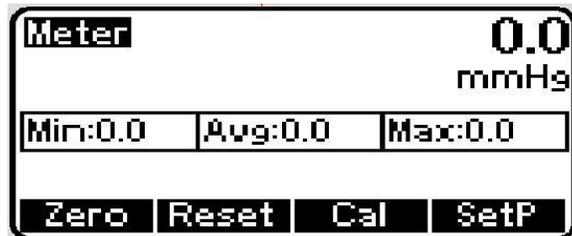
3. [VSM] Press the “Up Arrow” button until 80 mmHg is selected, and then settles at a slightly lower pressure level. Wait 10 seconds for the pressure to stabilize
