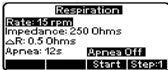
10. [AccuSim] Using the “Right/Left/Up/Down Arrow” buttons to change each values accordingly:
