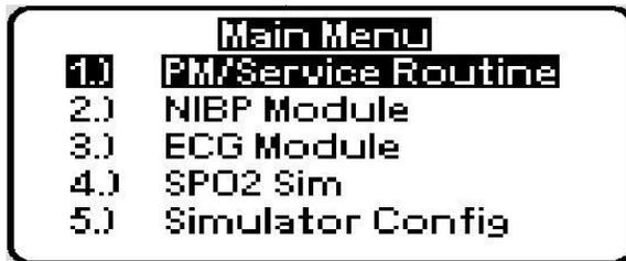
10. [AccuSim] Press “Scroll up/down” button to navigate to “PM/Service Routine” and press “Enter”
