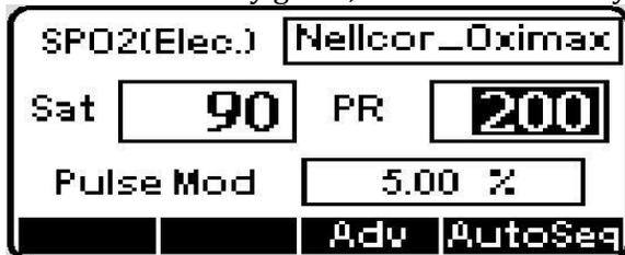
19. [AccuSim] Using the “Up/Down/Left/Right Arrow” buttons to navigate to “Sat” and “PR” and set the values accordingly:
