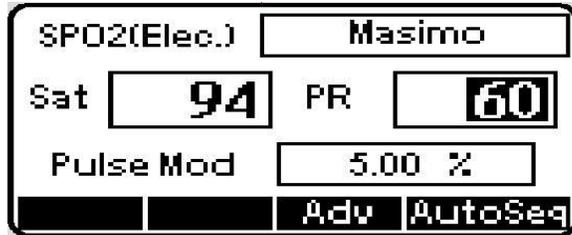
22. After Propaq stabilizes, verify that the following results are accurate [Pass/Fail]
