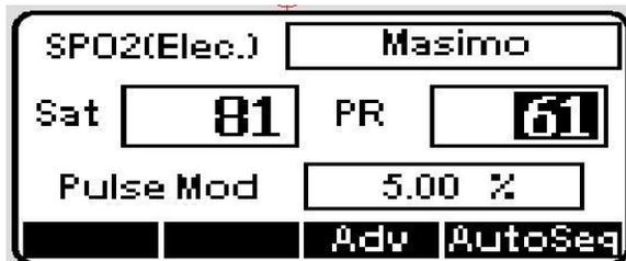
18. [CVSM] Verify that Saturation level is 81% ±3% and Pulse Rate is 61 bpm ± 1 bpm [Pass/Fail]
