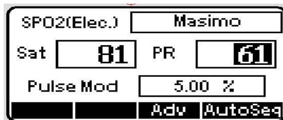
12. [VSM] Verify that Saturation level is 81%  $\pm$ 3% and Pulse Rate to 61 bpm  $\pm$  1 bpm [Pass/Fail]
