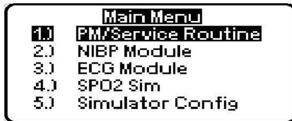
4. [AccuSim] Using the “Scroll Up/Down” buttons navigate to “PM/Service Routine” and Press “Enter”
