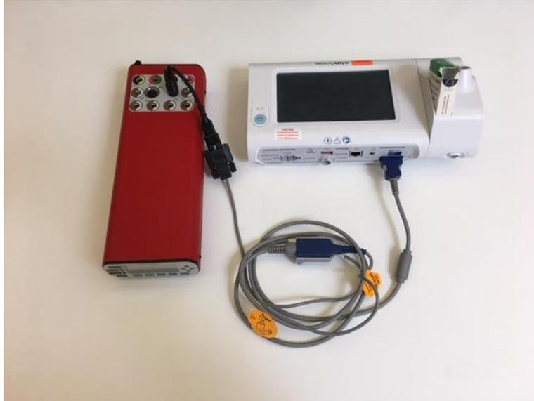
1. [AccuSim] Connect the “SPO2 Adapter” to the AccuSim simulator
