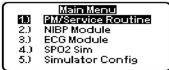
15. [AccuSim] Using the “Scroll up/down” button to select the “PM/Service Routine” and press “Enter”
