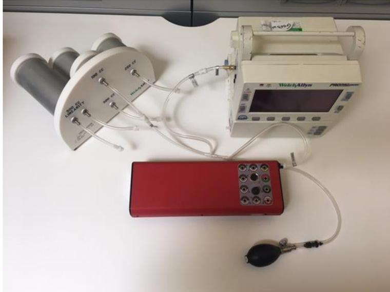
1. Connect the “NIBP Barb to Hose” hose to each cylinder (100cc, 250cc, 500cc, and 500cc Linearity) on the Test Volume
