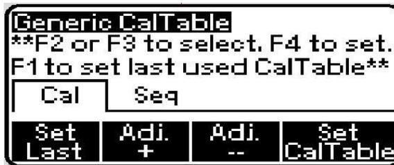
17. [AccuSim] Using the “Up/Down” button to navigate to “Spot LXI” and press “F4” to set the CalTable
