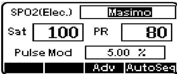
7. [AccuSim] Using the “Up/Down Arrow” button to change the Spo2 system to the current system being used
