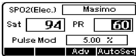
14. [VSM] Verify that Saturation level is 94%  $\pm$ 4% and Pulse Rate to 60 bpm  $\pm$  4 bpm [Pass/Fail]
