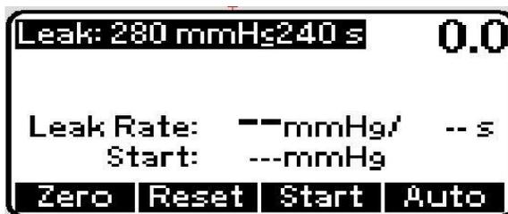
25. [AccuSim] Press “F2” to reset after finishing the test
