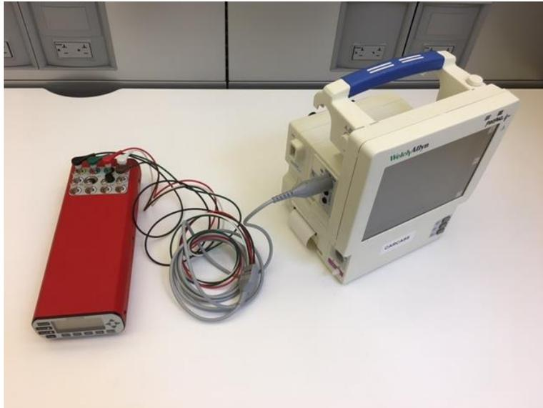
1. [AccuSim] Connect all ECG banana plug to AccuSim
