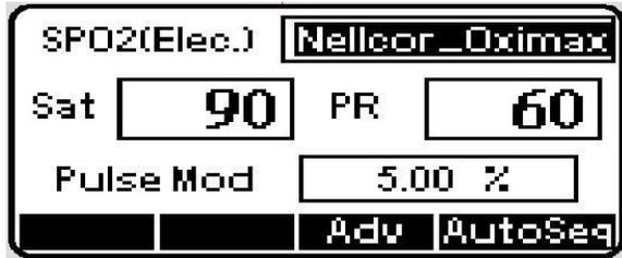
15. [CSM] Verify that Saturation level is 90% ±1% and Pulse Rate is 60 bpm ± 1 bpm [Pass/Fail]
