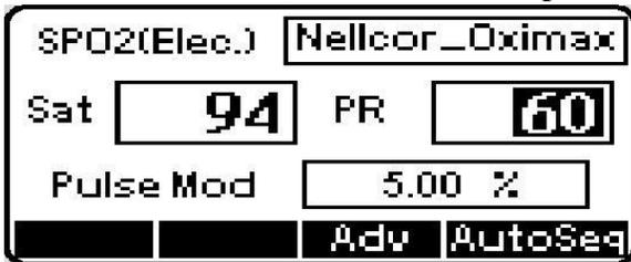
10. [Propaq] Verify that Saturation level is 94% ±4% and Pulse Rate is 60 bpm ± 4 bpm [Pass/Fail]
