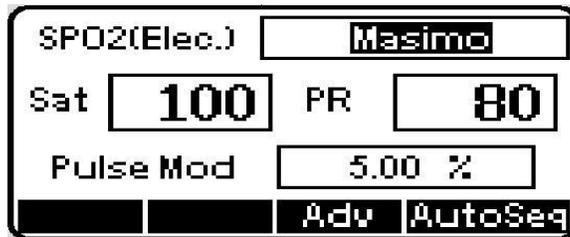
8. [AccuSim] Using the “Up/Down Arrow” button to change the Spo2 system to the current system being used
