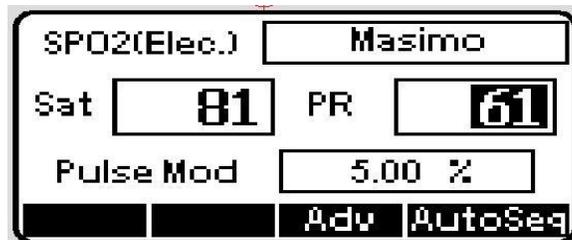
13. [LXI] Verify that Saturation level is 81% ±3% and Pulse Rate is 61 bpm ± 1 bpm [Pass/Fail]
