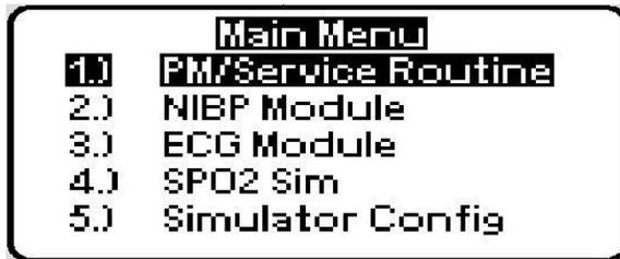
6. [AccuSim] Using the “Scroll Up/Down” buttons navigate to “ECG Module” and press “Enter”
