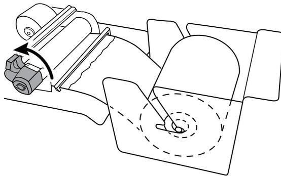
5. Insert the paper through the paper guide slot, and make sure it goes under and around the black roller bar.
