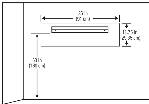
3. Affix the mounting rail bracket to three studs at the selected height using the available screws.
