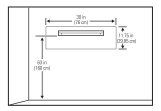
3. Affix the mounting rail bracket to two studs at the selected height using the available screws.
