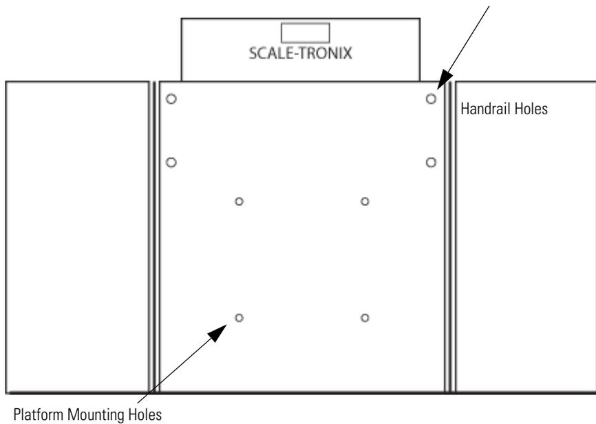
1. Position the weighing deck so that the two sets of holes under the flaps are closest to the mast.
