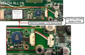
When replacing the LCD in a device that was manufactured after June 2014, there will be no inverter board installed. The LED Power Cable will plug directly into connector J107 (as shown).
