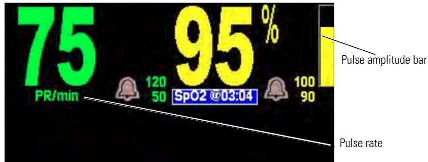
**Note** The pulse amplitude bar can help determine a correct SpO<sub>2</sub> sensor placement. This bar indicates physiological pulse activity, but is not directly related to pulse volume.
