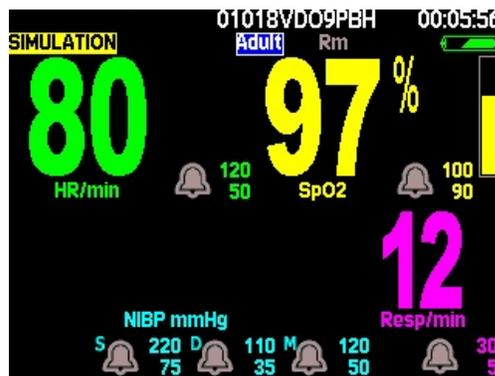
The monitor generates an alarm within seconds of reading this new set of simulated vital signs. The red alarm indicator (Figure 28) illuminates and flashes, the numerics for all violating vital signs—HR, SpO<sub>2</sub>, and Resp—turn red and flash, and the highlight moves to the most recent alarming numeric.
