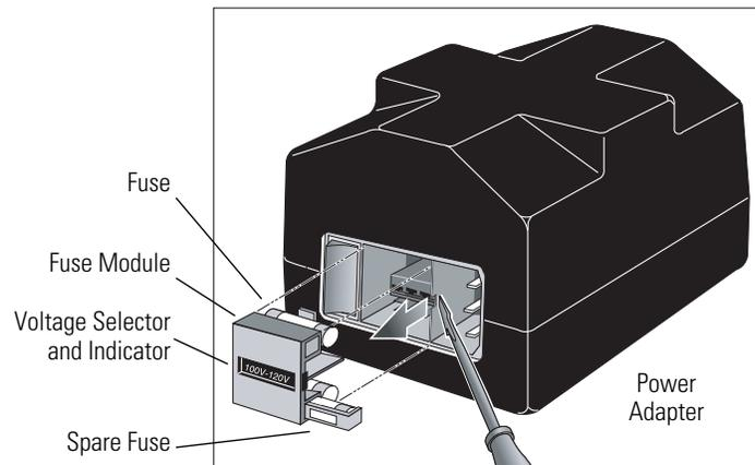
2. Using a small, flat-blade screwdriver, carefully pry the fuse module away from the adapter.
