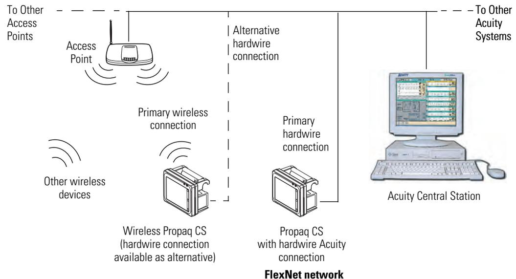
While connected to the network, the Propaq CS sends patient data to Acuity. Acuity continuously analyzes the data and provides appropriate alarm or alert messages at the Central Station and other network devices such as a hallway message panel or the Propaq CS itself. Acuity also stores the patient data for viewing or report printing.
