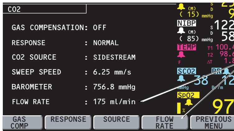
**FLOW RATE** is displayed only for sidestream CO<sub>2</sub> (not mainstream CO<sub>2</sub>).
