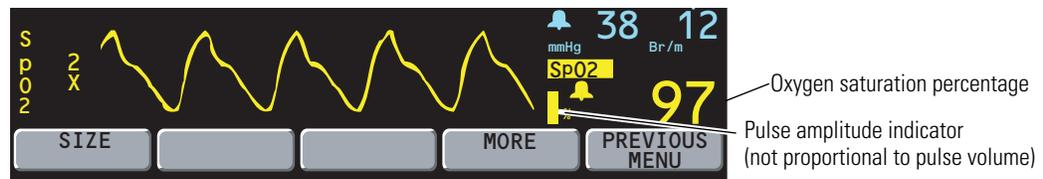
5. Press **SIZE** to adjust the waveform size for best viewing (1x, 2x, 4x, or 8x).
