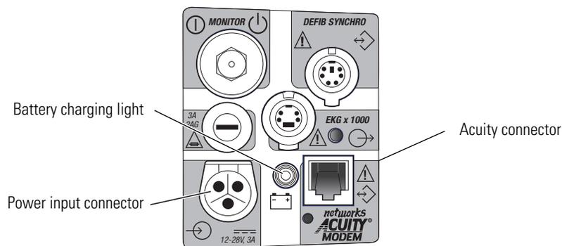
4. Connect the ac power adapter to the monitor and the wall outlet to charge the battery. Check to see that the green battery charging light on the monitor's right side panel is on.
