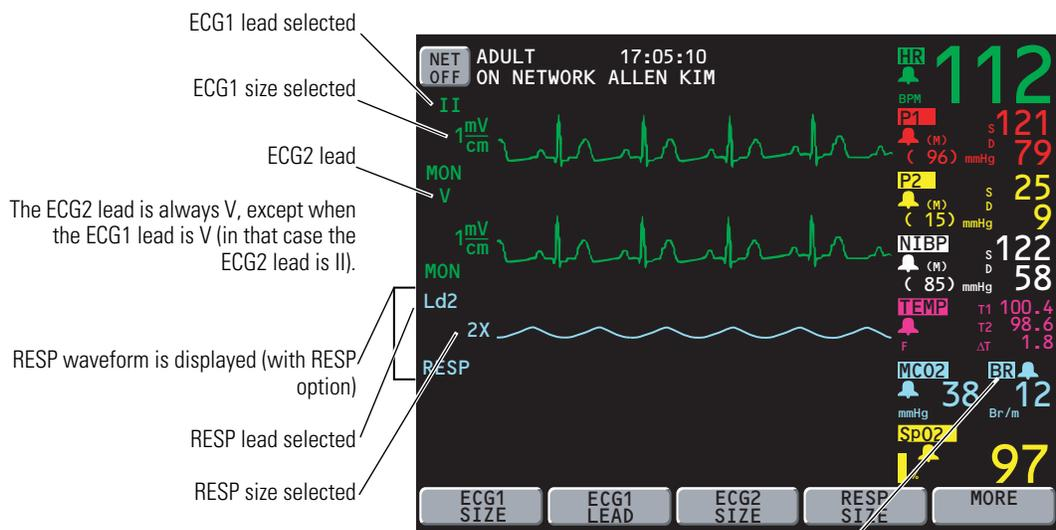
**BR** indicates respiration rate is derived from active CO<sub>2</sub> channel.
