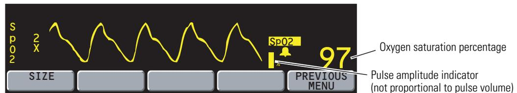
4. Press **SIZE** to adjust the waveform size for best viewing (1x, 2x, 4x, or 8x).
