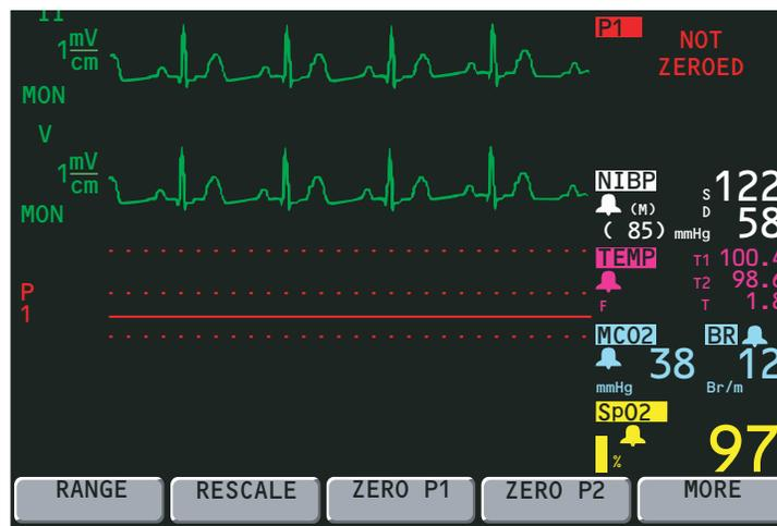
The message NOT ZEROED immediately appears in the IBP numerics window for the invasive pressure channel being used.
