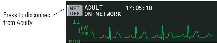
1. To disconnect the Propaq CS monitor from the Acuity network, press the **NET OFF** key on the upper left corner of the monitor display. (From the Main Menu you can also press **SETUP, ACUITY, NET OFF**.)
