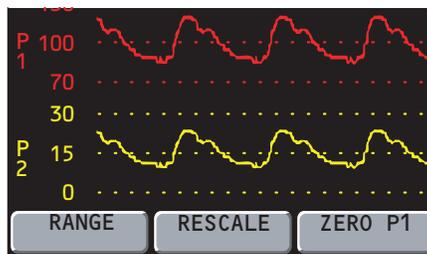
Whenever you press **RESCALE**, the monitor automatically adjusts the scale for the best appearance based on the highest and lowest pressure levels.
