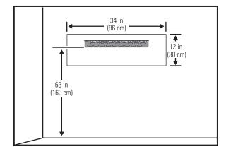
3. Affix the mounting rail bracket to two studs at the selected height using the available screws (anchors are provided for additional support).
