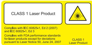
**Sensor recognition:** Designates the class of the installed laser product for distance measurement according to IEC 60825-1, Edition 2 (2007-03) and IEC 60825-1, Edition 3 (2014).
