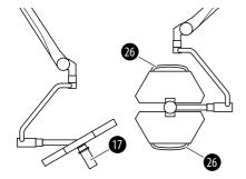
Hold the surgical light at the handle [17] or the side handles [26] and move it to the desired position.
