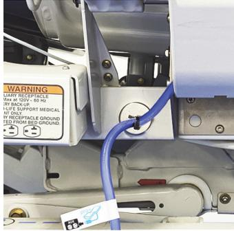
16. Plug the mattress power cord into the auxiliary outlet.
