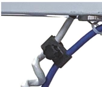
15. Route the power cord between the lower frame and headboard support.
