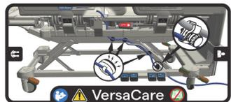
The surface power cord has magnets installed on the cord. The power cord is routed along the patient-left side of the bed to the head end of the bed. Below is an overall view of the cord routing; the numbered detail views correlate with Step 12 through Step 16 that follow.
