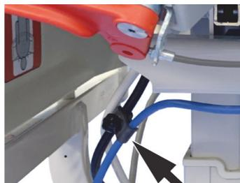
16. Route the power cord between the lower frame and headboard support.
