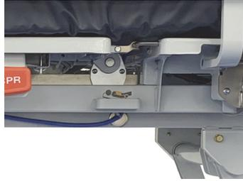
15. Attach one cord magnet to the upper frame, under the head section on the triangle bracket.
