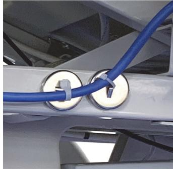
14. Attach one magnet to the upper frame below the head section on the head-end side of the siderail mount.
