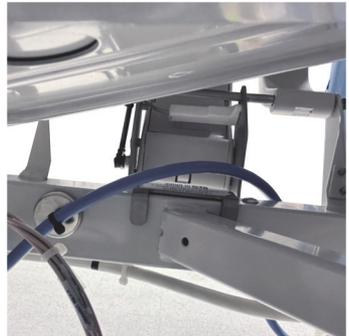
15. Attach the second cord magnet on the outside of the intermediate frame, between the siderail center arm and left side siderail weldment.
