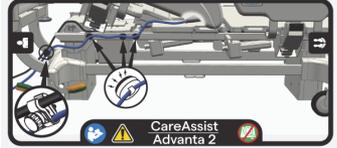
The surface power cord has magnets installed on the cord. The power cord is routed along the patient-right side of the bed. Below is an overall view of the cord routing; the numbered detail views correlate with Step 12 through Step 16 that follow.
