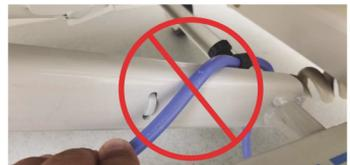
16. Route the power cord under the lift arm weldment, and between the head-end casters.
