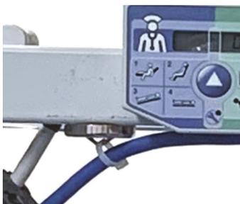
14. Put the straight section of the bed power cord into the cord clamp that is on the surface power cord. Use the knob to tighten the cord clamp.
