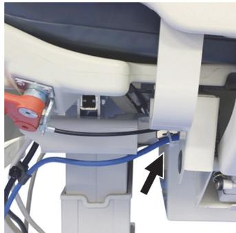
15. Put the bed power cord into the cord clamp that is on the surface power cord. Use the knob to tighten the cord clamp.
