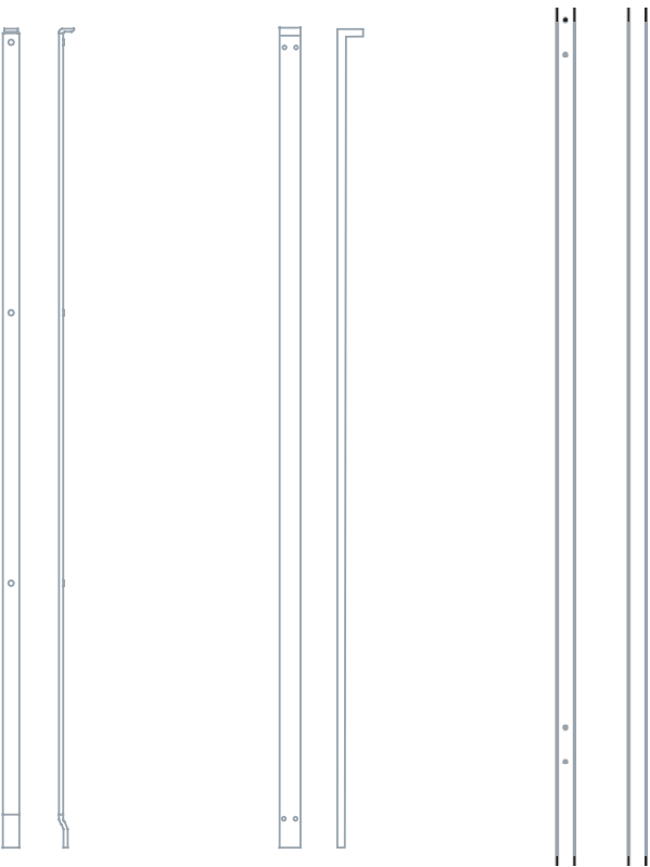
Slimline Upright Support: Max Load 272 kg / 600 lbs Standard Upright Support: Max Load 363 kg / 800 lbs Steel Upright Support: Max Load 500 kg / 1100 lbs
