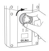
Reset the emergency stop by turning the button in the direction indicated by the arrows.
