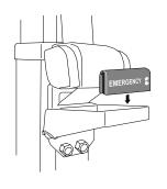
11. Press the tag marked "Emergency" securely into place on the emergency lowering device.
