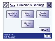
Select Ventilation Setting, Alarm Limits, Breath Timeout, or Source Gas.
