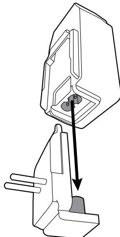
2. Slide the wall plug or line cord onto the transformer until it is firmly seated.
