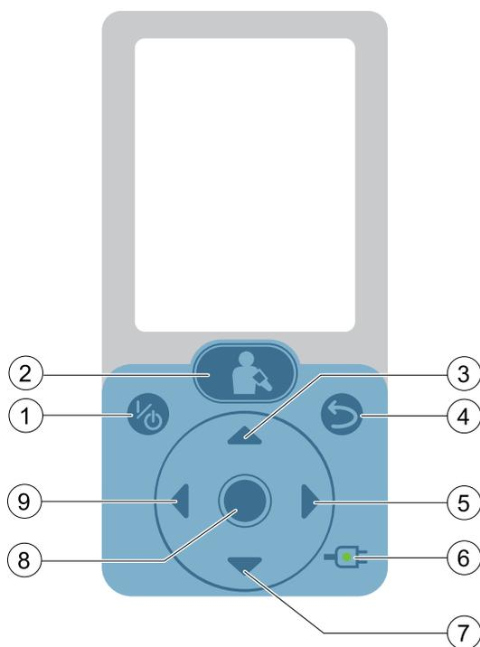
1. **Power on/standby** button: controls power to the device.
