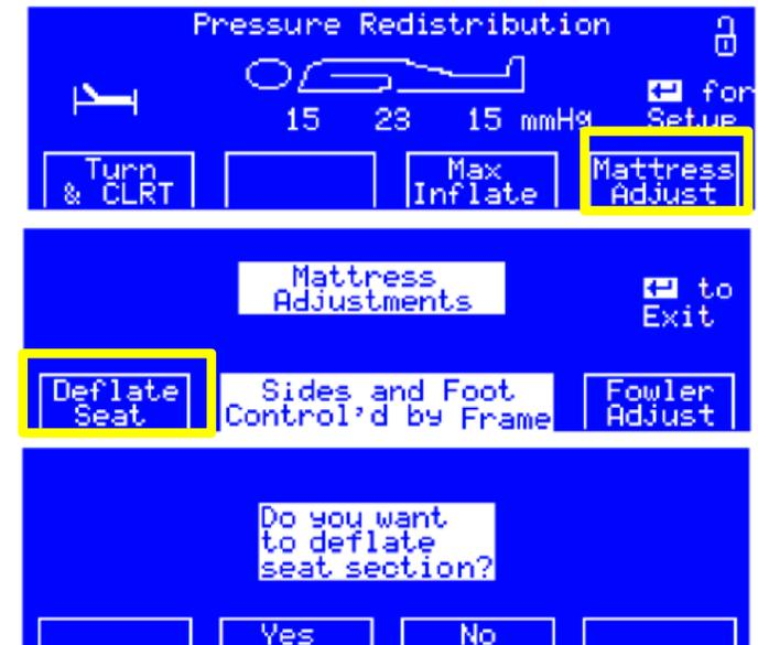
Seat deflate will remain active for up to 30 minutes. One minute before the Seat Deflate times out, an audible alarm sounds with the options to exit or continue for another 10 minutes.
