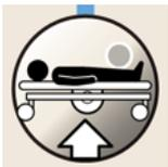
**NOTE:** You cannot zero the scale or weigh a patient when in transport mode. If you attempt to arm, a triple beep alert will sound and the raise bed indicator light will flash. Remove bed from transport mode by pressing and holding the raise bed indicator until single audible confirmation beep sounds. Bed exit is ready to be armed.
