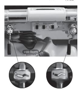
2. Turn the handle counterclockwise until the section is at the applicable height.
