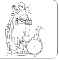
In raised position the SeatStrap loses its load and can easily be pushed to the side to facilitate toilet visits, for instance.
