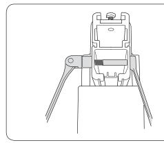
7. Mount the stop bolts in the rail ends, as illustrated.
