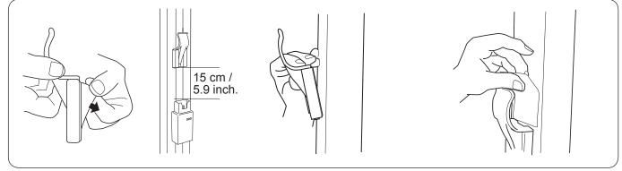
Remove the protective film from the double-adhesive tape on the parking bracket.
