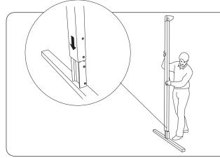
1. Turn the base so that the holes will align with the holes on the upright support. Mount the upright support on the base.
