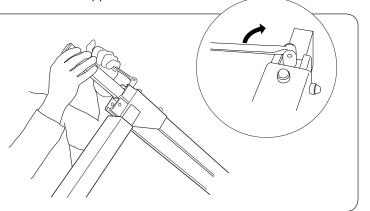
8. If support arms are to be used, do as follows: Insert the support arm into the upper part of the rail. Secure the support with the screw on the top of the locking rail (see 6. B).
