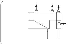
3. Remove the cover caps from the screws on the corner/locking rail and stop bolt on one end of the rail.
