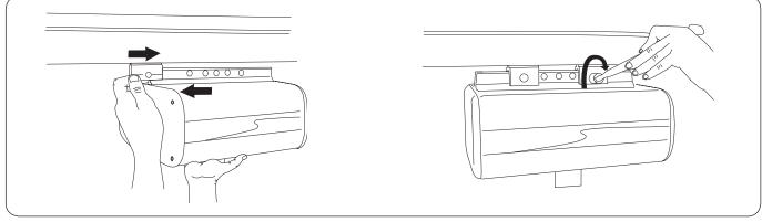
Loosen and remove the nuts and bolts from the rail carriers. Guide the lift unit onto one of the rail carriers. Use the nut and bolt provided to secure the rail carrier to lift unit via the outermost hole in the mounting rail on the top of the lift unit. Guide the other rail carrier onto the lift unit's mounting rail and align it with the outermost hole. Use the nut and bolt provided to secure the rail carrier to lift unit via the outermost hole in the mounting rail on the top of the lift unit.
