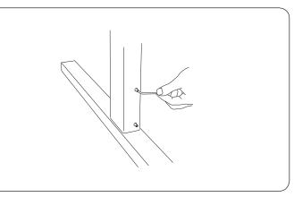
2. Affix the upright support to the base with the screws provided (2 on each side of each upright support, 4 screws per upright). Repeat steps 1 and 2 with the other upright support and base.
