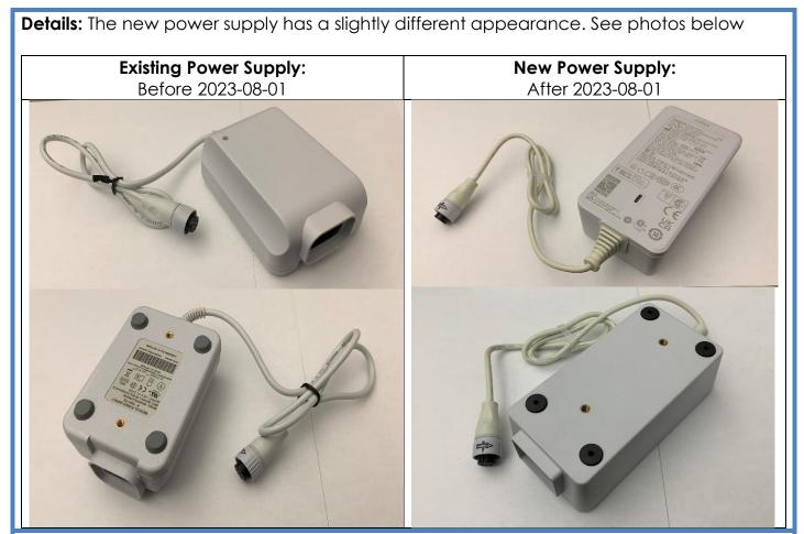
**Action:** No action needed. This bulletin is intended for clarification only. The new power supply is functionally identical to the existing supply and is backwards compatible with all intended CSM devices and approved mounting solutions in service centers and the field.
