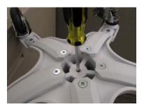
3. Using a 5mm Allen key and pliers (or similar tool set), loosen the bolt by turning in a counter-clockwise direction, as shown below. This may be difficult because of the thread-lock used in production of the stand. Loosening the bolt will push the base and pole apart.
