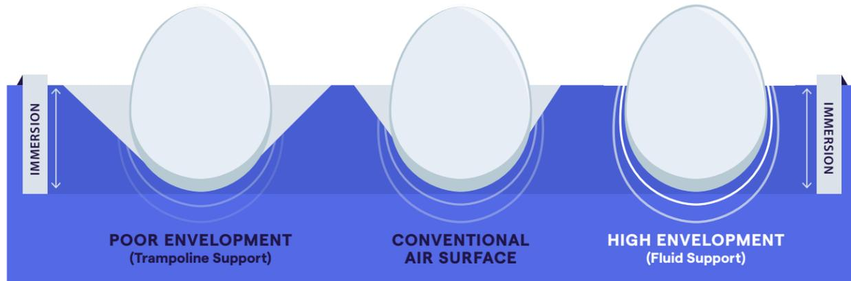
**Figure 1:** Identical Levels of Immersion (penetration depth into the surface) but different levels of Envelopment (conformability and contact area). LEFT: Trampoline-like support (Poor Envelopment) such that pressure is concentrated at the apex, increasing Peak Interface Pressure. RIGHT: Fluid support (High envelopment); pressure is broadly distributed across the contact area and peak pressure is minimized.
